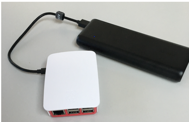
Figure 2: The SpeakUp Box (a SpeakUp server running on a Raspberry Pi low cost single board computer).
